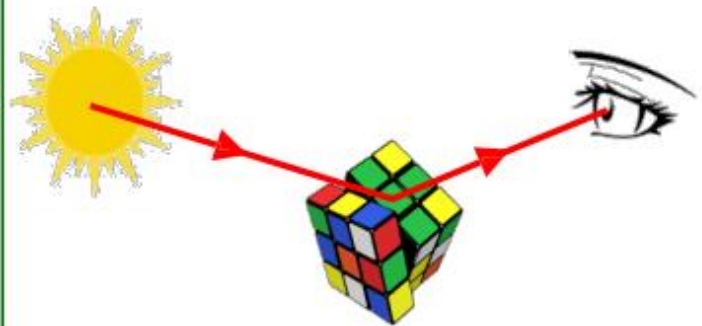
Here the light goes from the light source, bounces off the object and into your eyes, so that you see the object.
